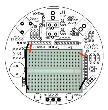
3. Zero ohm jumpers make good jumpers for the prototype board. Use 22 gauge solid hookup wire for making longer wires.
