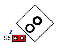
S5 is the connected to the un-configured RCA connector J2. The right pin of S5, Pin 1, is connected to the center pin of the RCA connector. The left pin of S5, Pin 2, is connected to the outer shield of the RCA connector.
