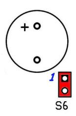
Connector S6 is used to connect the piezo sounder to a circuit in the breadboard area. The top pin of S6 is wired to the + terminal of the piezo sounder. The bottom pin of S6 is wired to the other terminal of the piezo sounder.
