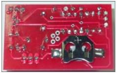
series. DO NOT POWER THE MAINE BUGS KIT WITH ANYTHING OVER 5 VOLTS! Battery voltages over 5 volts can destroy the microprocessor chip. It is best to remove the coin cell and power the kit from a 3AA battery pack or 5 volt supply when on the bench in order to maximize coin cell life.
