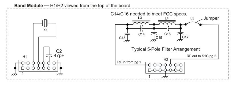
5-Pole Filters: All capacitors pF, Kemet 5% C0G or equiv.
