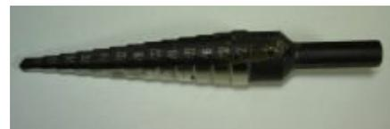
The step-drill cuts pretty clean holes in thin metal tins! One bit drills many different sized holes...
