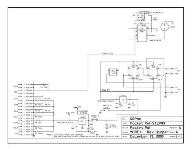
OK. Now its time for some microprocessor fun! The Picaxe micro in the Pocket PAL is used as an audio signal generator and as a frequency counter. For this step, we will only be concerned with the audio signal generator.
