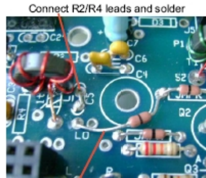
Connect jumper from jumper to LO hole
