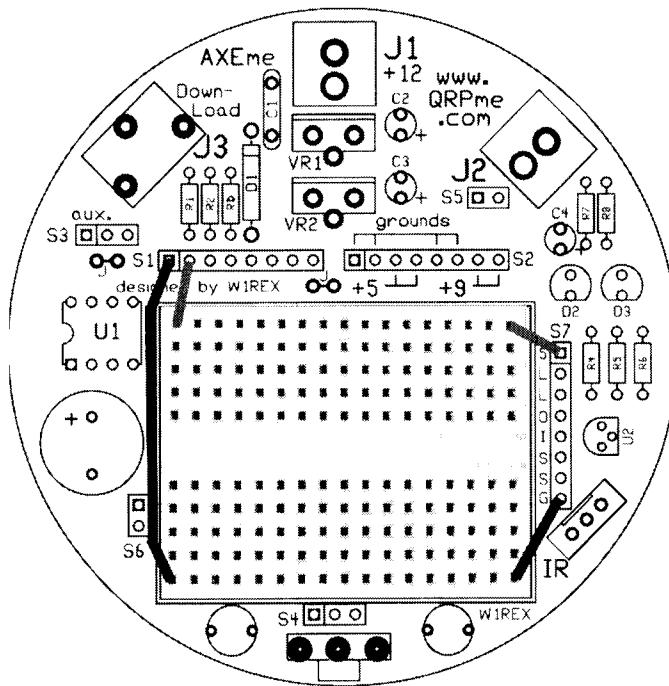
Or use the top left corner for +5V and the top right corner for +9V.
