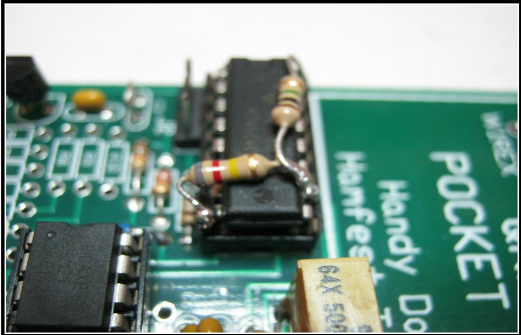
5. A pair of biasing resistors are required for the ripple counter chip to clock properly. I soldered them VERY carefully directly to the pins of the counter chip.
