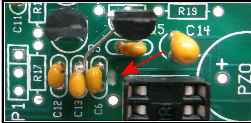
1. Cut the +5V feed to the collector of Q5 where it passes around U1, the Picaxe micro. Just to the left of the DIP socket, the trace passes underneath C6 and then on to the collector of Q5.
